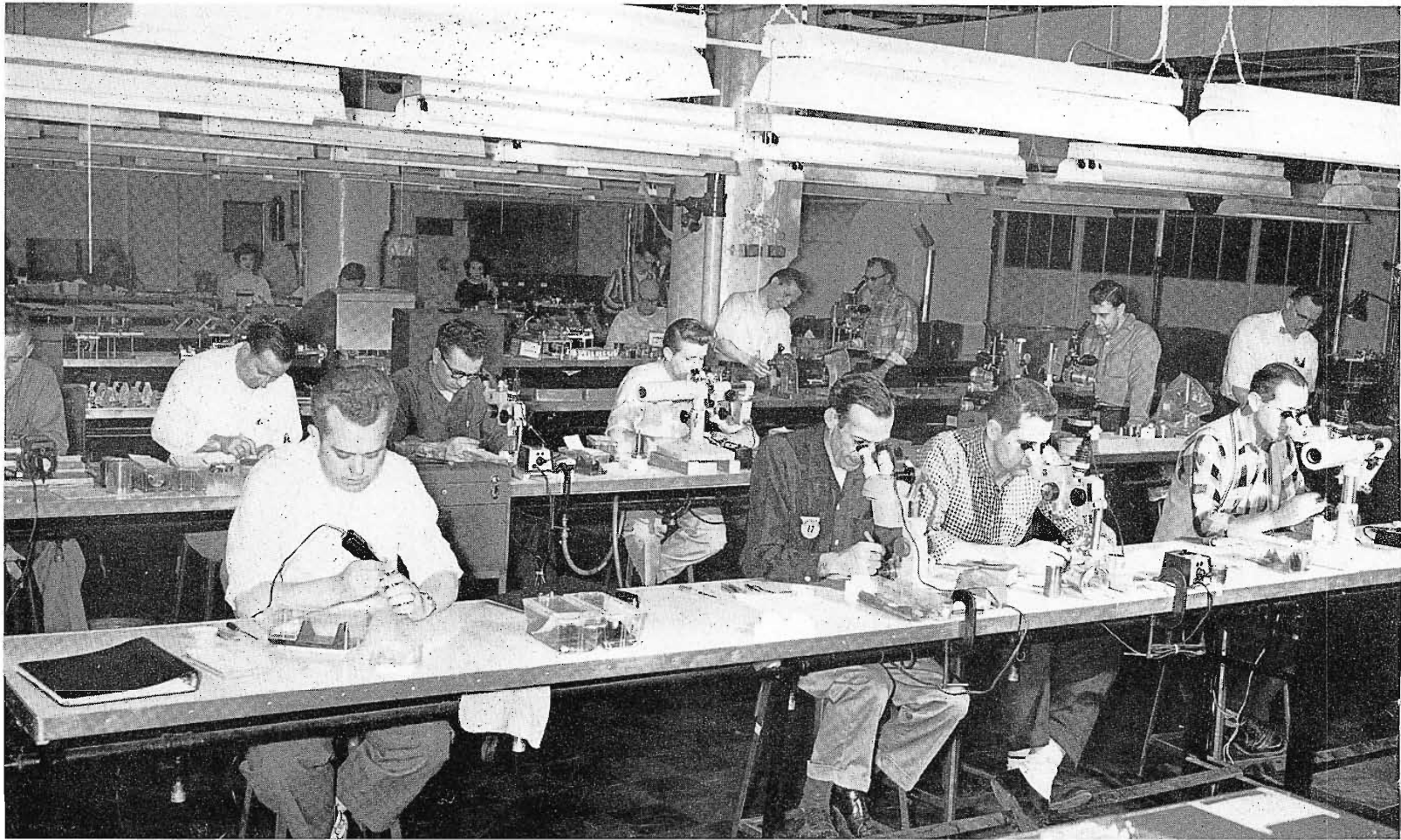
FIG. 1. These skilled technicians are assembling headwheels for TV Tape. Individual attention is given to each assembly; one technician follows each headwheel through all stages of its assembly, alignment and test. He positions heads in the headwheel with respect to pole-tip protrusion, tracking, quadrature and balance.
