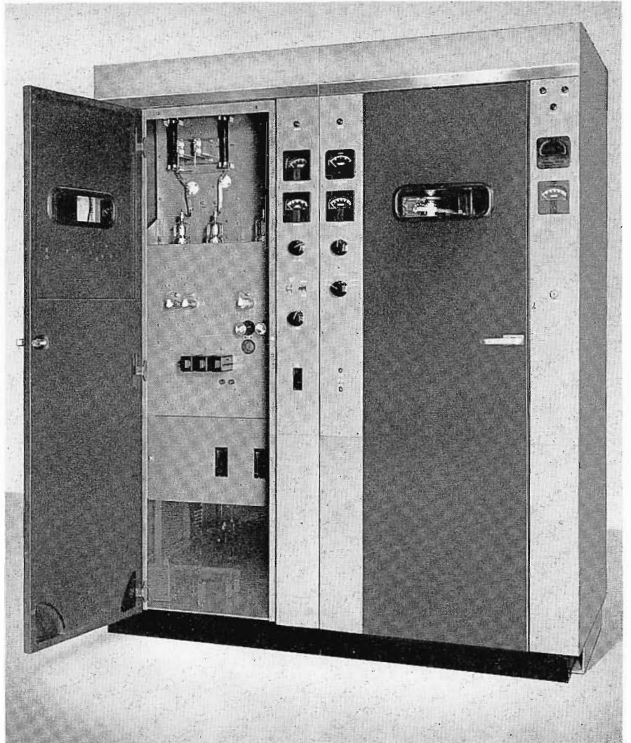
FIG. 3. The exciter and IPA stages are shown here. Note the three crystal sockets on the exciter chassis, and the easy to reach tubes.
