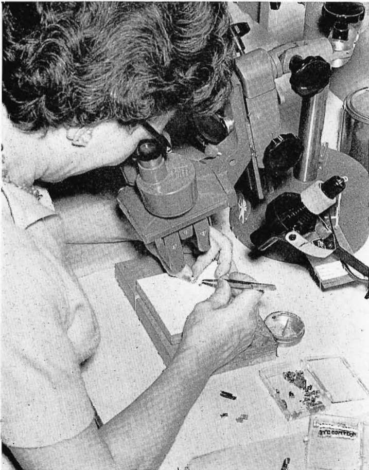
FIG. 5. Here, pole tips are being inserted and cemented into head blocks prior to machining. This is the initial stage of head fabrication. Two of these blocks are joined together in the following process to form a single video head.
